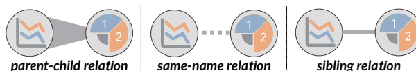
Fig. 7: The visual encodings of three types of relations in the insight graph of the Colinsight system. A line with varying thickness indicates the parent-child relation. A dashed line indicates the same-name relation. A straight line indicates the sibling relation.
